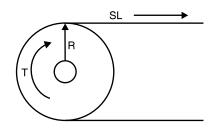
If the load above requires torque T pound-inches and is driven with a pulley on the motor shaft a with a radius of R inches, the side load imposed on the motor shaft is T/R pounds. If the motor shaft is connected to a sprocket for a chain drive, R is one half the pitch diameter of the sprocket. If an external load with a weight of W pounds is also being supported by the motor shaft above, the total side load on the shaft is:
