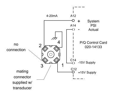
Wiring diagram for 2-Wire pressure transducer, 788-50035, when supply voltage UB does not exceed 30 volts.
