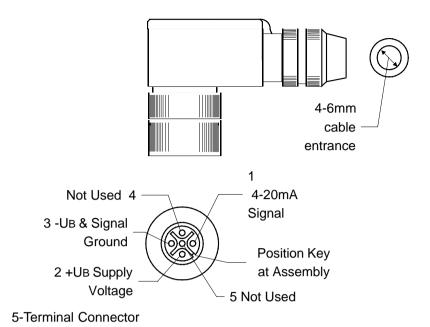
167-011106-8 Mating Connector for Valve-Spool Position Transducer
