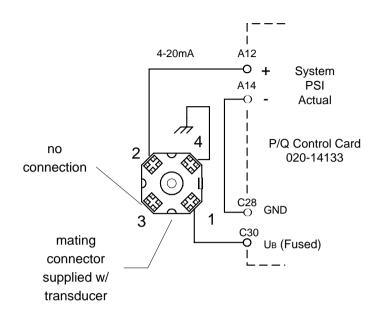
Wiring Diagram for 2-Wire pressure transducer, 788-50035, when using an isolated power supply.
