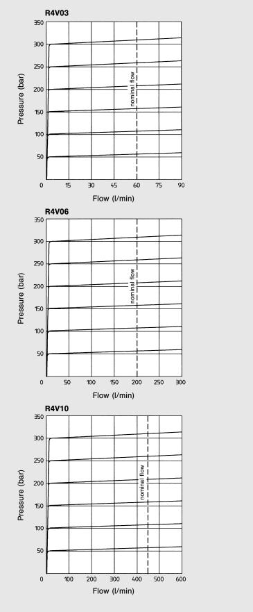
min. pressure setting  $\ge 3$  bar (depending on flow and viscosity). Fluid 40 cSt at  $50\,^{\circ}\text{C} \pm 0.5\,^{\circ}\text{C}.$
