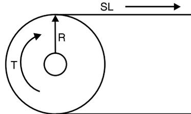
If the load above requires torque T pound-inches and is driven with a pulley on the motor shaft with a radius of R inches, the side load imposed on the motor shaft is T/R pounds. If the motor shaft is connected to a sprocket for a chain drive, R is one half the pitch diameter of the sprocket. If an external load with a weight of W pounds is also being supported by the motor shaft above, the total side load on the shaft is:
