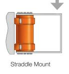
The upper portion of the bracket is bolted to the shaft flange, the lower portion is bolted to the endcap flange.
